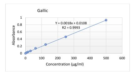
Fig 1: Gallic Acid Calibration curve
