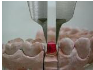
Figure 2 The sliding calliper with customised jaws to facilitate measurement of the mesiodistal crown diameter
