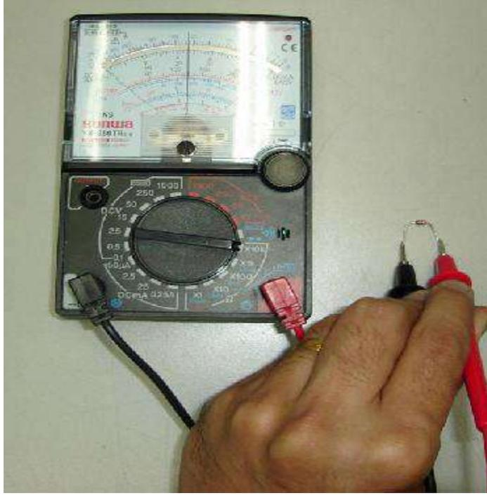
Use analogue multimeter to test Zener diode
