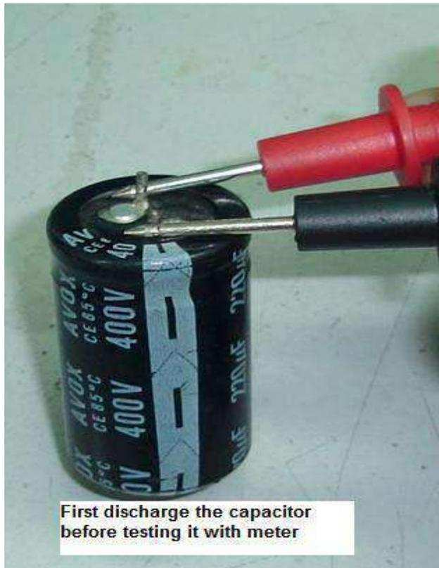
First discharge the capacitor before testing it with meter
