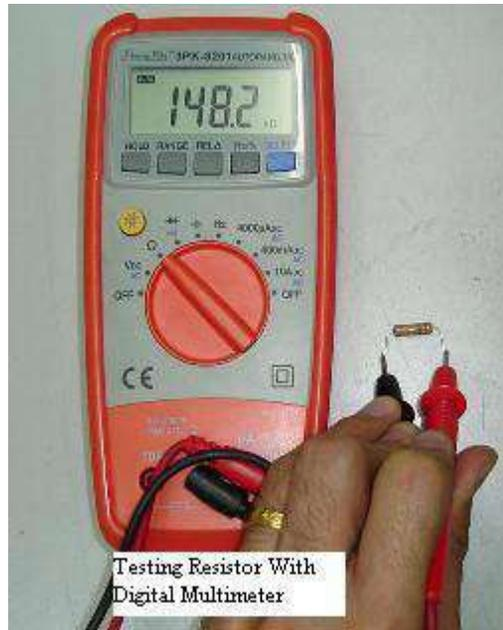
Testing Resistor With Digital Multimeter
